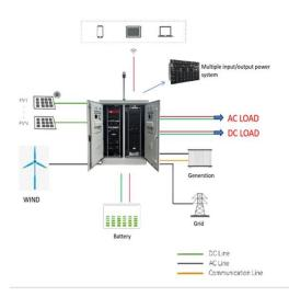
supports max 4 sets of 215kWh IBS215K1KC battery cube access to achieve max 860kWh battery energy capacity. Max 4 sets can work in parallel ...
