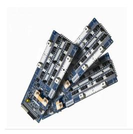
technology dedicated to the oversight of a battery pack, which is an assembly of battery cells, electrically organized in a row x column matrix ...
