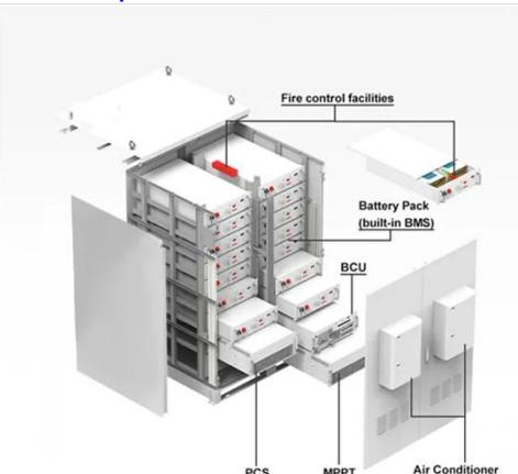
system (BESS) is well defined by its name. It is a means for storing electricity
