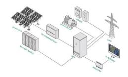
combing battery energy storage and EV charging to reduce costs, increase capacity and support the grid.
