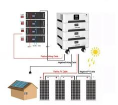
Manufacturer Outdoor cabinet energy storage system is a compact and flexible ESS designed by Megarevo based on the characteristics of small C& I loads.
