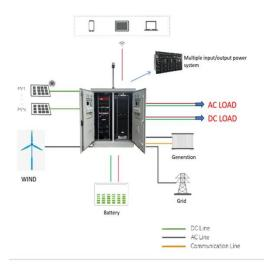
Energy storage systems (ESS) can store power from any generation source, such as solar panels, a generator or the utility grid itself. That power can be used immediately to run ...
