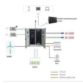
The Containerized energy storage system refers to large lithium energy storage systems installed in sturdy, portable shipping containers, which usually range from 5ft, 10ft, 20ft, and 40ft, and
