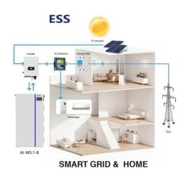
three-in-one modular design combining solar power generation, energy storage, and backup power supply. With ...
