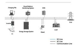
stabilize the photovoltaic output, and a photovoltaic storage system microgrid of a 5G base station is ...
