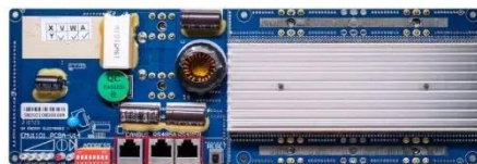
RS485 Communication between battery and inverters Baud rate: 9600bps RS485 Interface Communication between parallel grids or EMS and PC Baud rate: 9600bps
