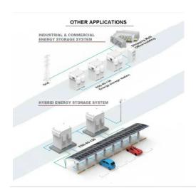
integrating solar PV, battery storage, diesel backup, and grid connectivity, prioritizing solar energy for daytime use with excess stored for ...
